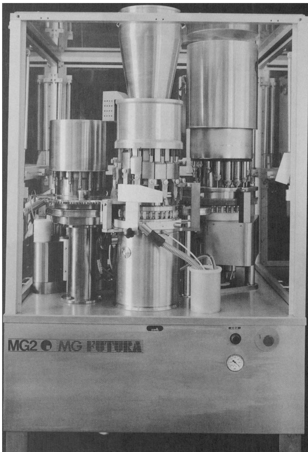
Fig. 12 MG2 Futura automatic capsule-filling machine. (Courtesy of MG America, Inc., Fairfield, NJ.)
